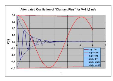
Here we have the typical behaviour of a model with a rather high mass-moment of inertia. While for the previous lower-weight F3J-model the fast pitching-oscillations already came to rest after about one cycle, here it takes about 4 - 5 cycles.
