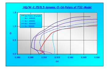
b. Usually the selection of distinct airfoils for a lifting wing is done by a comparison of the performance of potential airfoils over the possible speed range given by the weight/unit-area. For manned gliders this at the end is given in form of a quasistationary velocity polar. In the first instance it requires that for all possible stationary velocities of the glider the corresponding lift, the airfoil-drag, the drag caused by interference of the airplane parts,
