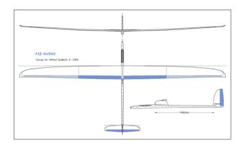
The left graphic shows the 3 side-draft for a new **F3J**-model designed by the author. Flight-mechanical characteristics of the model as given below have been determined by means of the "*FMFM*"-program (*Elight-Mechanics for Elight-Models*) which is described in more detail on the homepage www.hq-modellflug.de.
