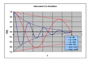
The left graphic provides a rough idea of the difference between the fast pitching-oscillations and the slow, damped c.g. oscillations.
