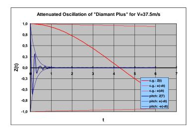
As we see, the fast pitchingoscillations very soon come to rest, whilst the c.g.-oscillations take a long time and can easily be balanced out by RC-control.
