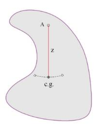
A simple practical method to determine the mass-moment of inertia of any given body is the following; If a body like that in the left graphic is equipped with an axis through A it can be stimulated to swing around this axis and the time T for one full period of oscillations is given by
