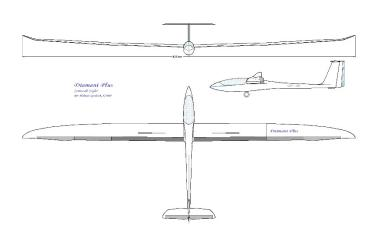
From the original "Diamant" the fuselage was used for practical reasons und thus the momentum-arm of the model was predetermined. In our home-page www.hq-modellflug.de one can find all details about the design aspects for the new development.
