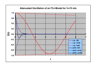
With increasing flight-velocity also the gliding-angle increases. As can easily be taken from the above formulae, the dampening constant  $\delta_{c,g}$  decreases slightly with increasing V and  $\vartheta$ , while the oscillation frequency decreases.
