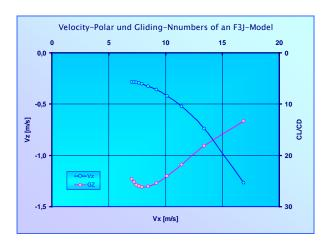
Finally, the left graphic provides the quasi-stationary theoretical performance parameters of the complete F3J-model for its expected operational flight range under inclusion of all sorts of drag related to the model.
